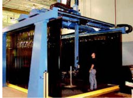
The automated ultrasonic inspection system checks aircraft wing sections using water squirters that transmit ultrasonic waves to detect defects.
