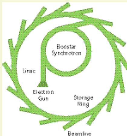
*Diamond is a third-generation 3 Giga electron volt synchrotron light source. It will use arrays of magnets called insertion devices to generate extremely intense, narrow beams of electromagnetic light for scientific experiments.*
