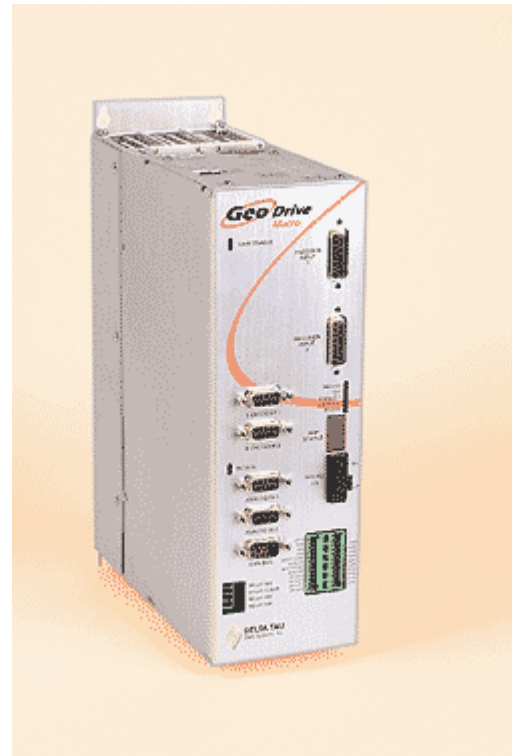
The Geo Macro drive communicates with a controller through a 125 Mbits/sec fiber-optic ring. The drive sends PWM, torque, velocity, or position commands and accepts a wide range of motor-position feedback. The one and two-axis servodrive amplifiers support a wide variety of motors, power ranges, and user interfaces.
