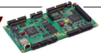
To meet the need for inexpensive, yet precise motion control, Delta Tau has launched the new Turbo PMAC2 "Clipper" controller. Communicating via Ethernet or RS-232, the multi-axis controller is very powerful but compact and cost-effective. It has a full Turbo PMAC2 CPU section and provides a minimum of 4 axes of servo or stepper control with 32 general-purpose digital I/O on a single board.
