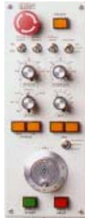
NC Operator Control Panel
